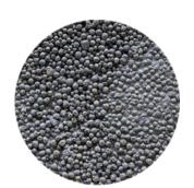
**Eco-cork lime:** A thermal insulation plaster made from natural hydraulic lime, which naturally absorbs CO<sub>2</sub> during curing. Combined with expanded cork granules, it offers high environmental performance and is a natural alternative for sustainable building envelopes.
